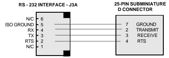
**Note:** The IBM computer normally has male RS-232 connectors so the modular adapter should have a female connector.
