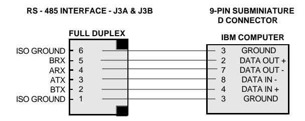
Another alternative for RS-485 is to use an RS-232 to RS-485 converter that plugs into the computer RS-232 receptacle external to the computer and is powered from a +9V DC wall plugin adapter. One such unit is the B & B Electronics Model 485OT9L.
